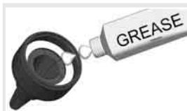
When using Uponor Standard expander heads extra grease needs to be applied in the interface between the tool and the expander head.
